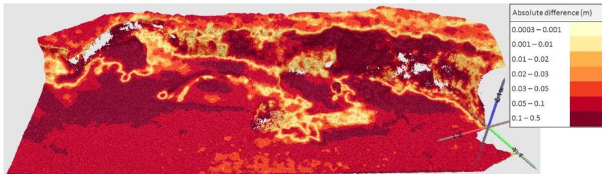
Figure 1. Absolute difference in UAV-MVS point clouds (of a 10 m section of coast) for 2010 versus 2013.
