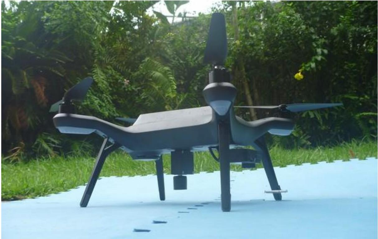
Figure **Error! No sequence specified.** The Specolo module mounted together with a GoPro camera on a Solo UAV from 3D Robotics.
