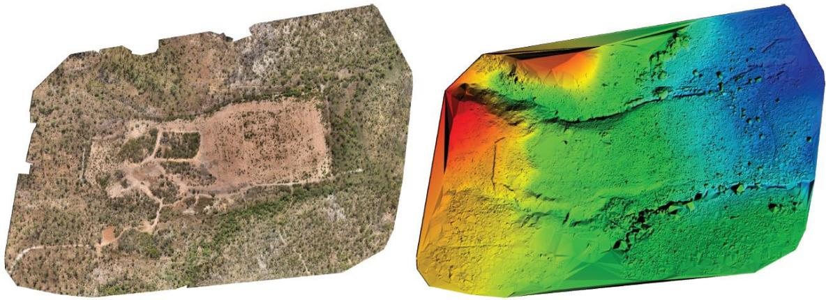
*Figure 1. Preliminary orthomosaic and Digital Surface Model (DSM) for the former Jabiluka mine site, created from 364 individual UAV images acquired on 10<sup>th</sup> July 2015.*
