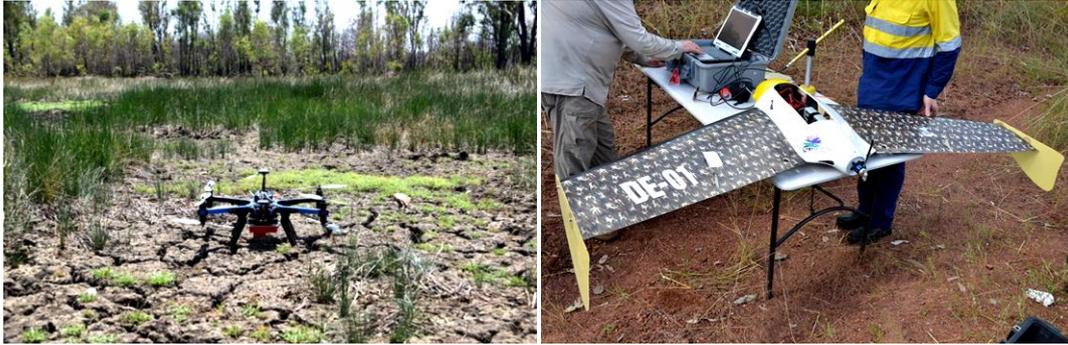
Figure 1. Left: X8 octocopter with MicaSense Red edge payload. Right: Swampfox X5 delta wing with Sony Nex5 cameras (R, G, B and modified NIR).
