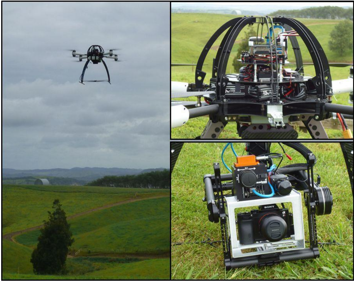
Figure 1. Custom build 'Aeronavics' small UAS with hyperspectral, thermal, and RGB camera payload.
