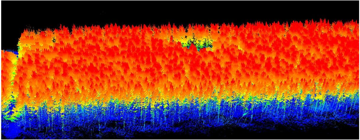
*Figure 1. An ALS point cloud over a mature Pinus radiata plantation derived from Scion's UAS*
