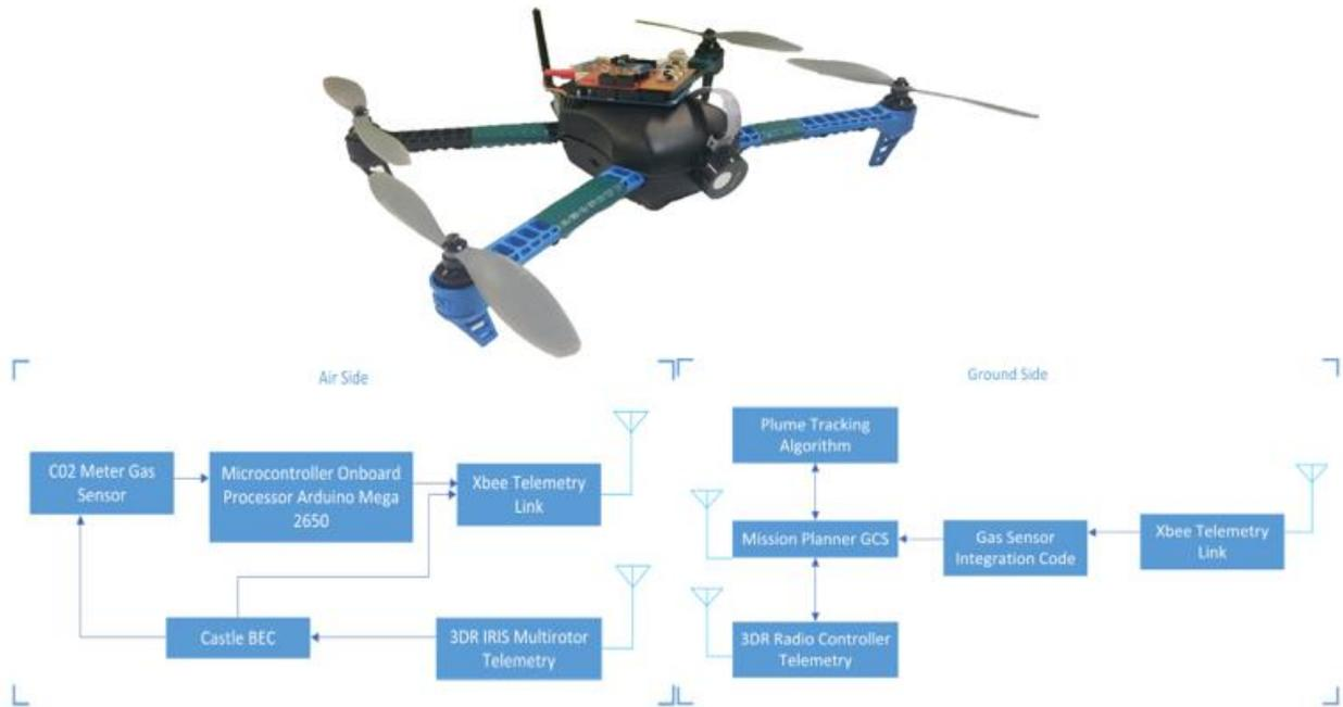
Figure 1. System Architecture with Flight System.
