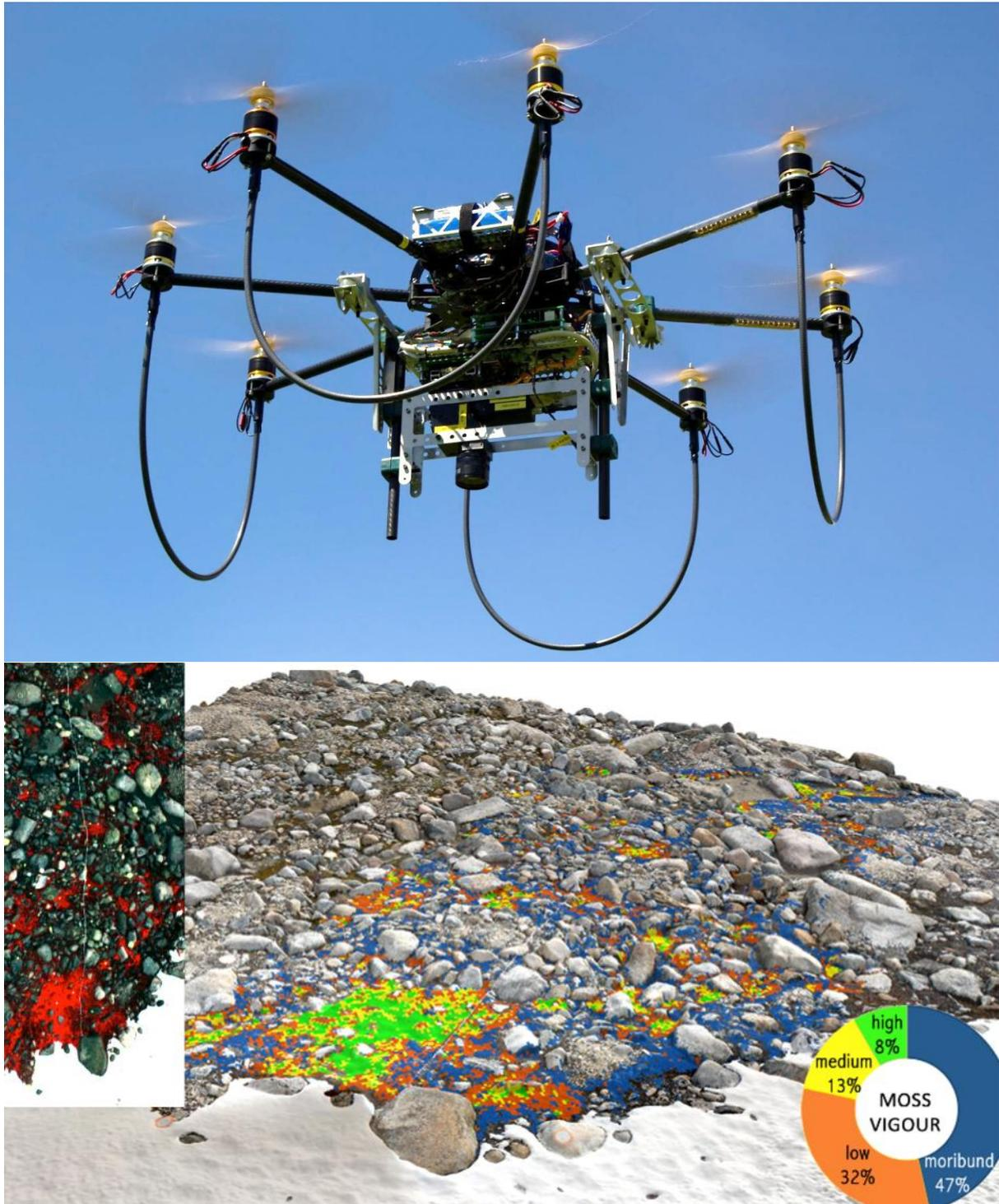
Figure 1. HyperUAS system carrying a pushbroom hyperspectral sensor (top); moss health derived from 162 spectral bands in the VNIR spectral range for an Antarctic moss bed.
